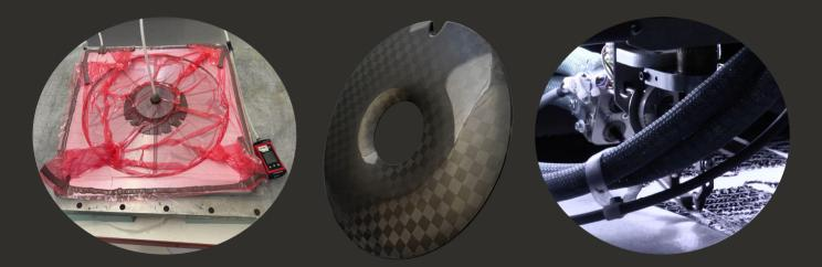
Resin infusion was selected to manufacture the prototype covers. This manufacturing technique allowed for a low cost high quality part to be produced with a short lead time. Covers were manufactured with different quantities of plies along with the TFP structure so that their performance could be compared against the baseline prepreg cover.
